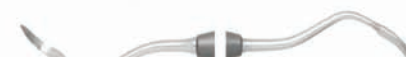
ED-025-315 Crane Kaplan #6 Mirror image blades that taper to a point from a 2.0mm width. The terminal shank is set at 35° to the handle with a reach of 15mm.
